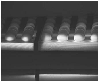
Plasma-diced bumped die on tape
